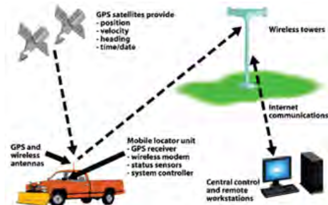
FIGURE 15 Schematic diagram of AVL system (Allen 2006).
