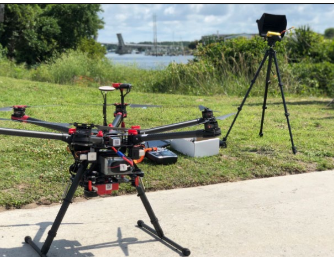
Above: Black Widow (DJI S900) drone used to collect project data.
