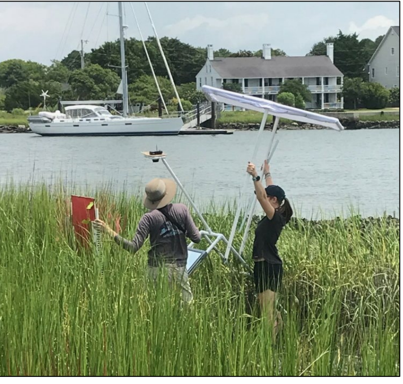
Above: Conducting vertical accuracy assessment with mirror apparatus.
