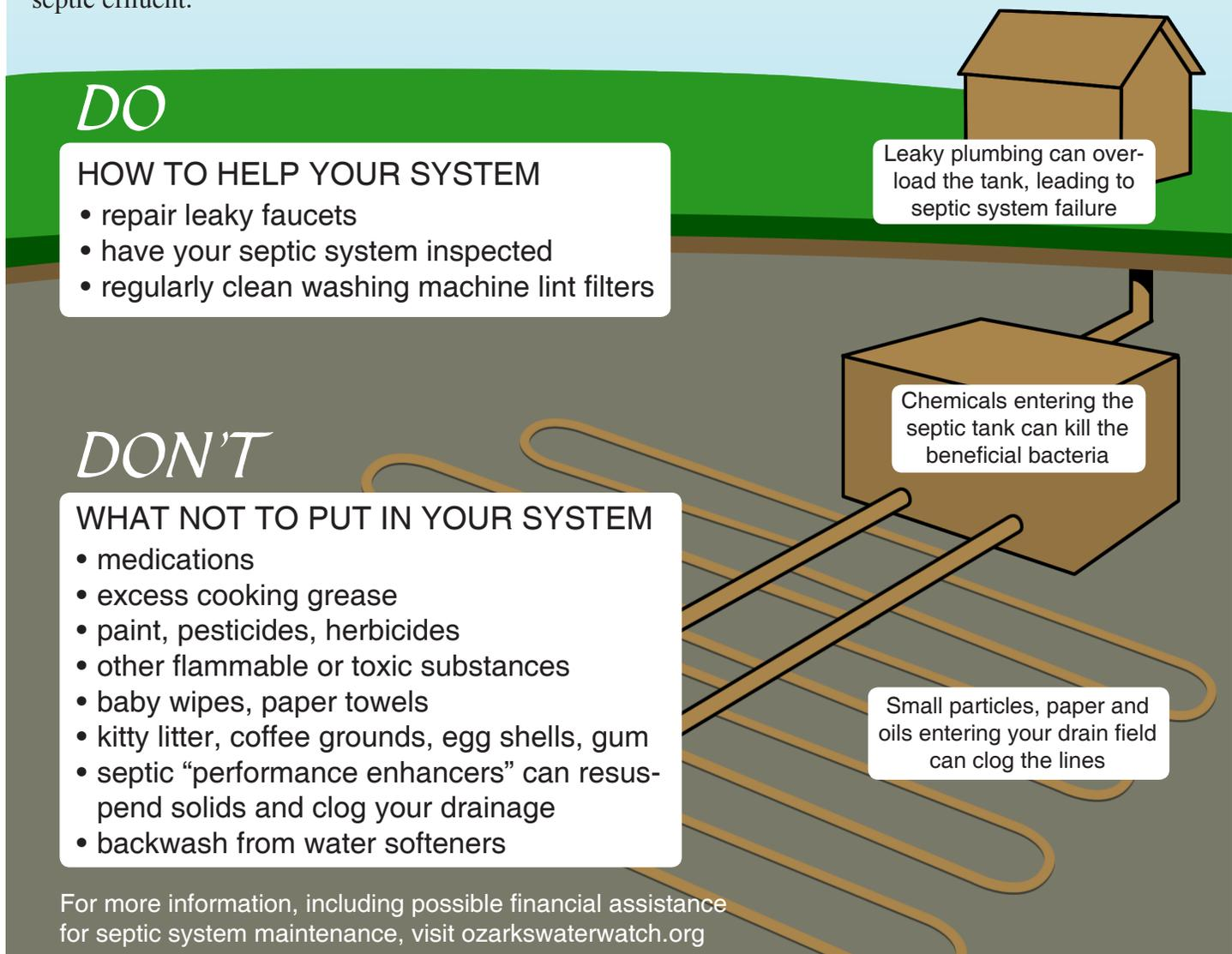
Leaky plumbing can overload the tank, leading to septic system failure
