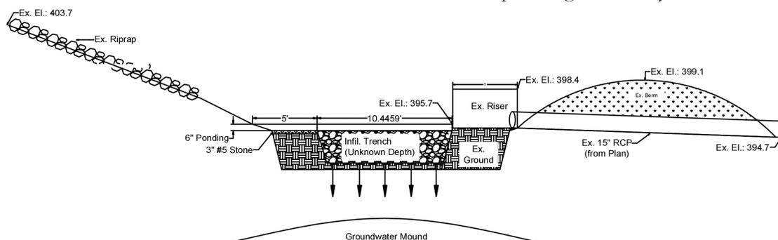
Figure 1: An example groundwater mound beneath an infiltration trench.
