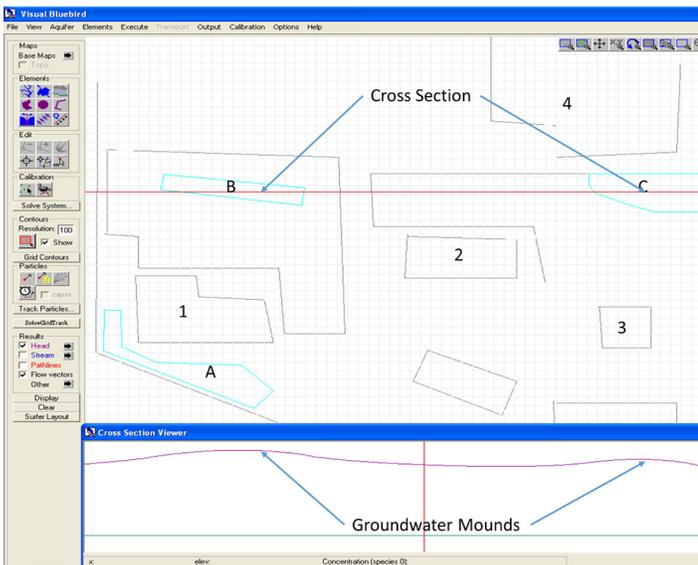
Figure 3: Cross section view of groundwater mounds considering infiltration areas B and C.
