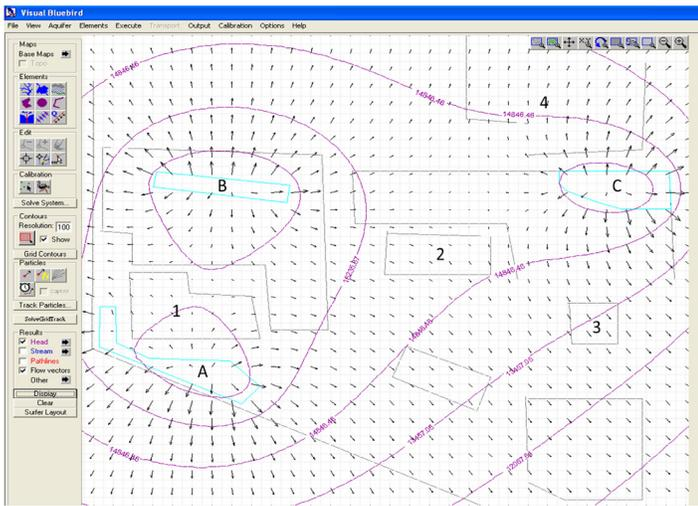
Figure 2: Flowlines with potentials (arrows indicate flow direction; longer arrows indicate higher flow velocity). This situation is considering infiltration from three sources. Numbers are buildings while letters are infiltration areas.
