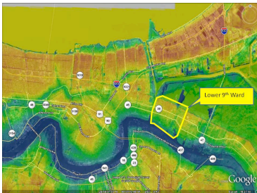
Figure 1. Generalized elevations in the city of New Orleans areas derived from light detection and ranging (LIDAR) imagery. The blue and green areas represent higher elevations (the Mississippi River was at 3.65 m stage during the LIDAR capture), whereas the yellows to reds indicate lower elevations, with much of these areas below sea level. Note the green ridges (Metairie and Gentilly ridges), which represent natural levees from old channels. Source: Data downloaded from Atlas: Louisiana Statewide GIS, http://atlas.lsu.edu .
