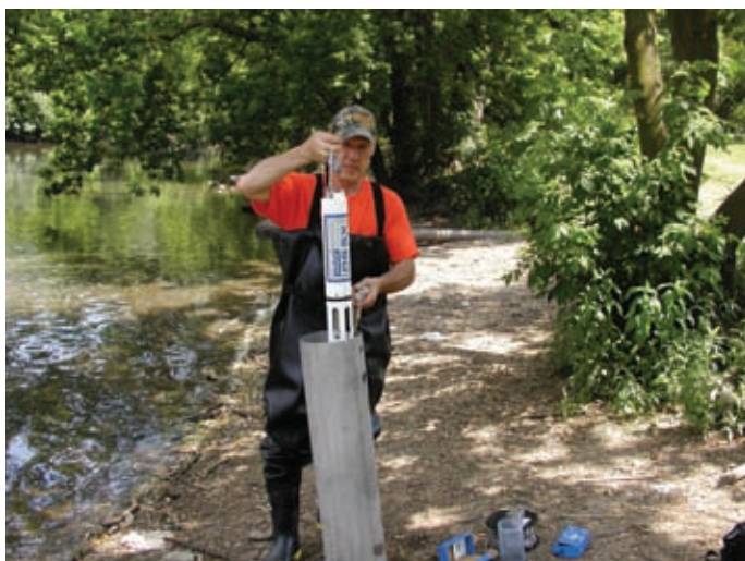
Figure 1. A technician from the City of Elmhurst, an agency member of the DuPage River Salt Creek Workgroup, retrieves a data logger from an instream casing on Salt Creek.
