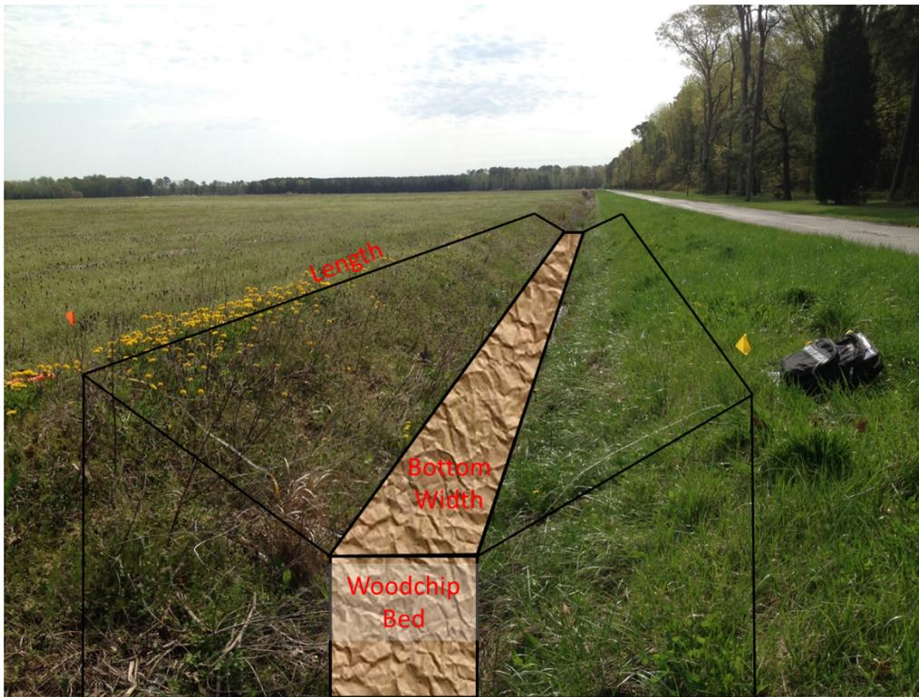
Figure 2. Potential to use woodchips to provide denitrification in ditches with minimal grade or with periodic connection to shallow groundwater.
